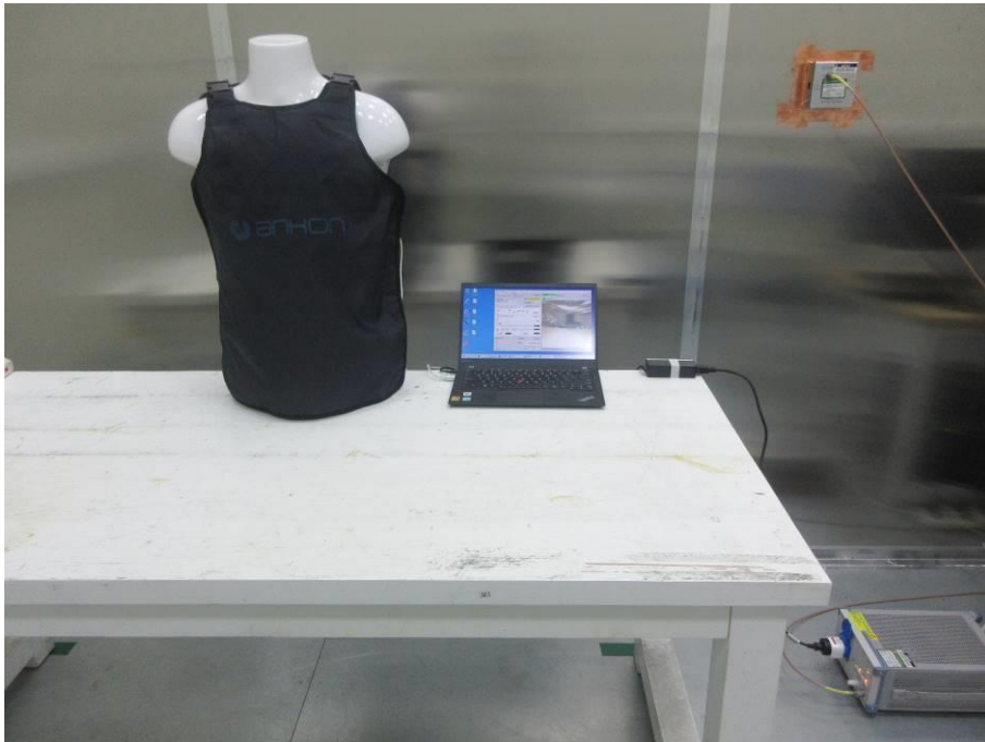
POWERLINE CONDUCTED EMISSIONS MEASUREMENT SETUP
