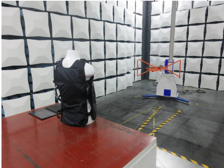
RADIATED RF MEASUREMENT SETUP (30MHz ~ 1 GHz)
