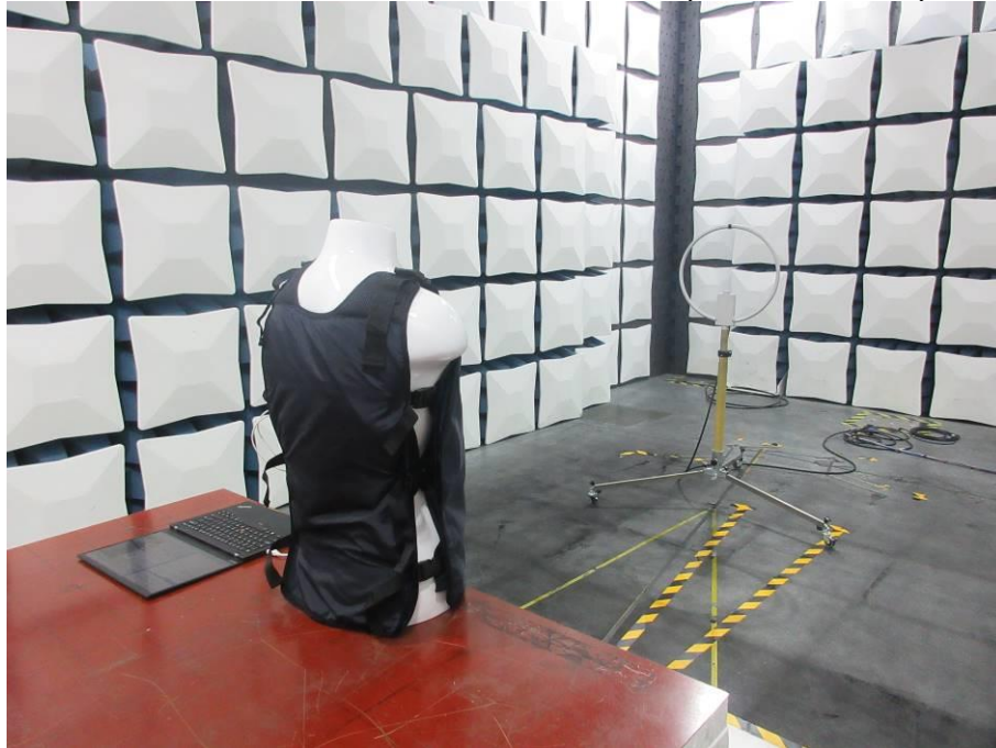
RADIATED RF MEASUREMENT SETUP (9KHz ~ 30 MHz)
