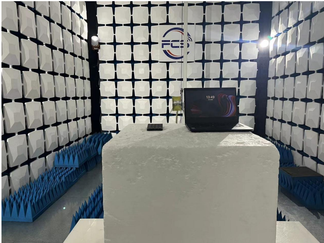
Above 1GHz for radiated emission test setup
