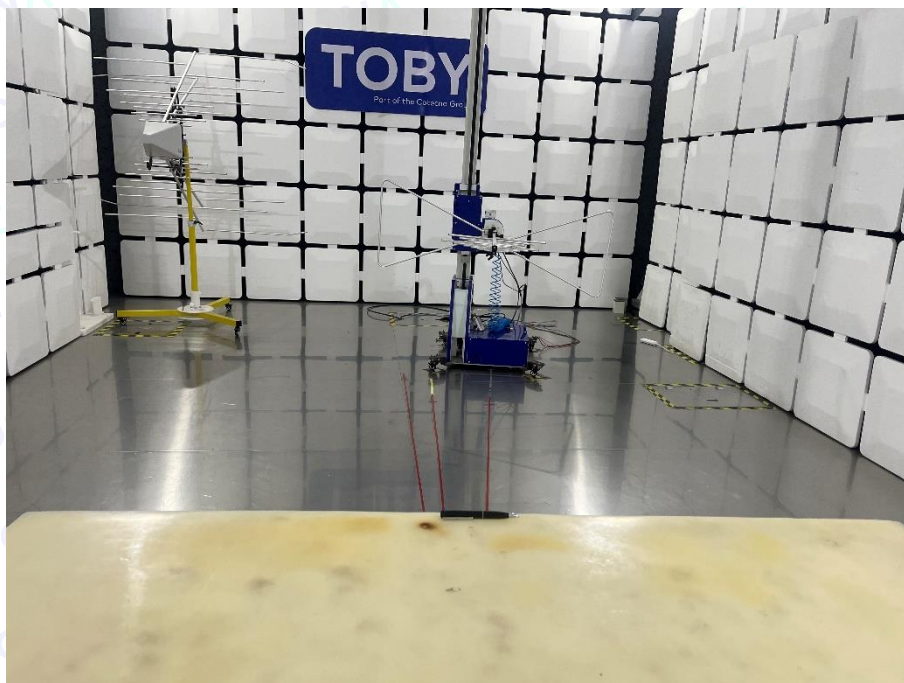
Photo of Setup for Radiated Emission (30MHz~1GHz)
