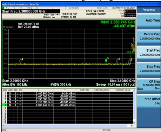
Left Band edge hopping on
