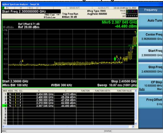
Left Band edge hopping on
