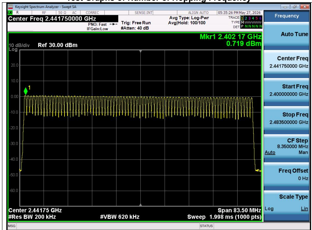
Test_Graph_BR_HOP_ANT1_NA_1Mbps_Number of Hopping
