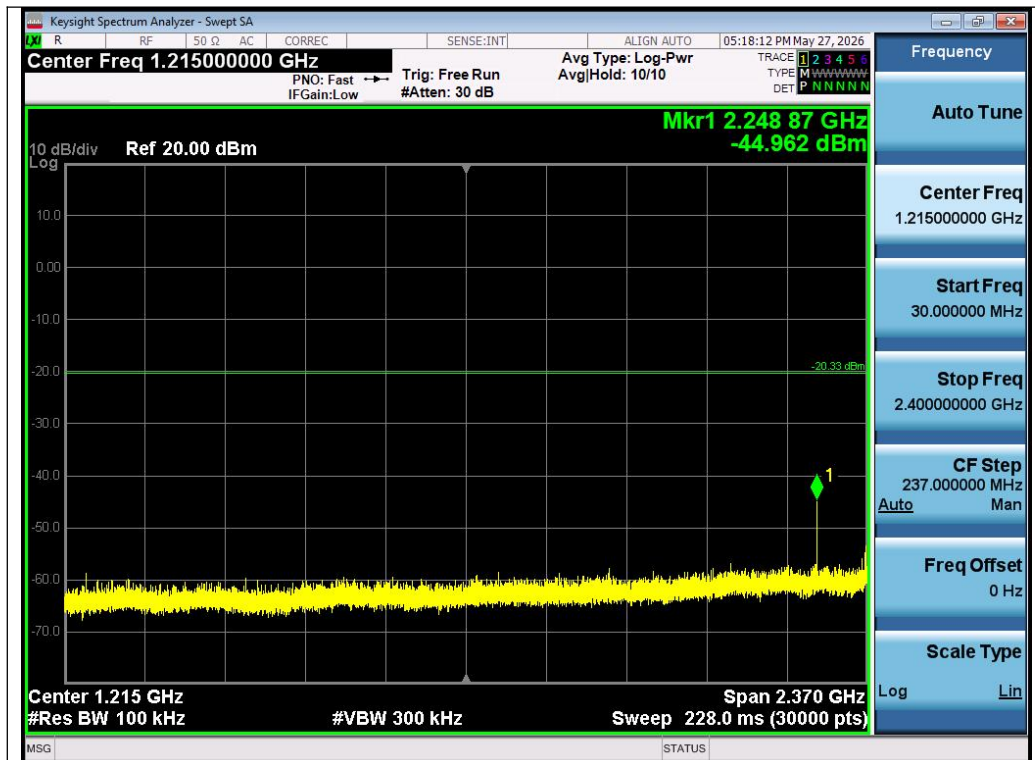
Test_Graph_EDR_ANT1_2441_3Mbps_Lower Band Emissions
