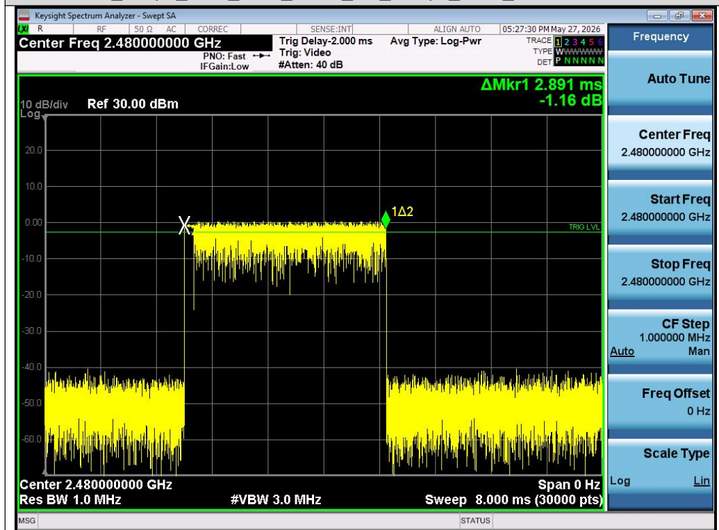
Test Graph EDR HOP ANT1 NA 3Mbps 2480 Time per Burst
