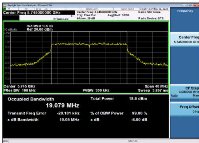
U-NII-3 6dB Bandwidth-802.11ax(20MHz) ,5745MHz,Ant9
