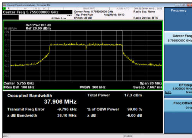
U-NII-3 6dB Bandwidth-802.11ax(40MHz) ,5755MHz,Ant9
