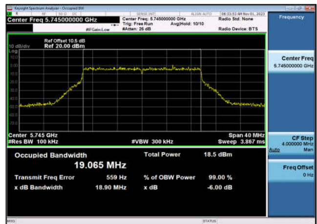
U-NII-3 6dB Bandwidth-802.11ax(20MHz) ,5745MHz,Ant10
