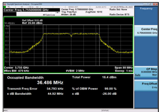
U-NII-3 99% Bandwidth-802.11ac(40MHz) ,5795MHz,Ant10
