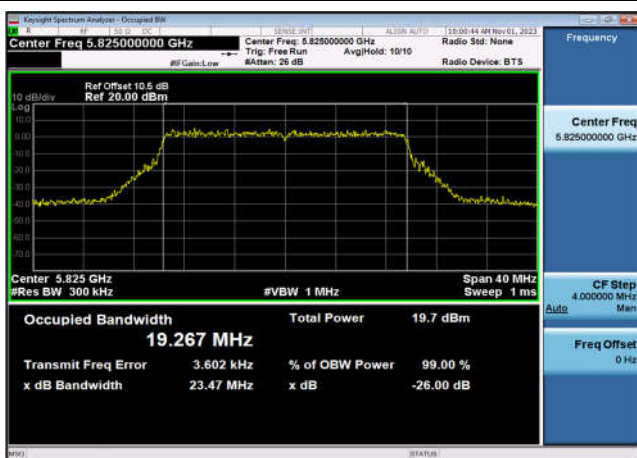
U-NII-3 99% Bandwidth-802.11ax(20MHz) ,5825MHz,Ant9
