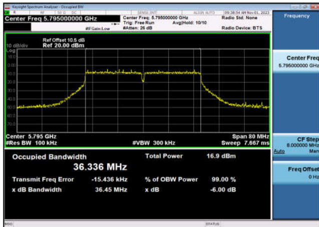
U-NII-3 6dB Bandwidth-802.11ac(80MHz) ,5775MHz,Ant9
