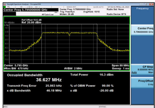
U-NII-3 99% Bandwidth-802.11ac(80MHz) ,5775MHz,Ant10
