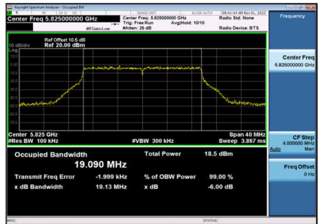
U-NII-3 6dB Bandwidth-802.11ax(40MHz) ,5755MHz,Ant10
