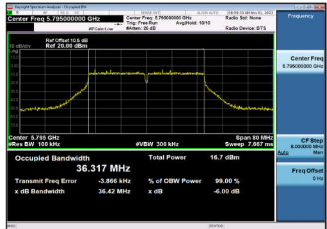
U-NII-3 6dB Bandwidth-802.11ac(80MHz) ,5775MHz,Ant10
