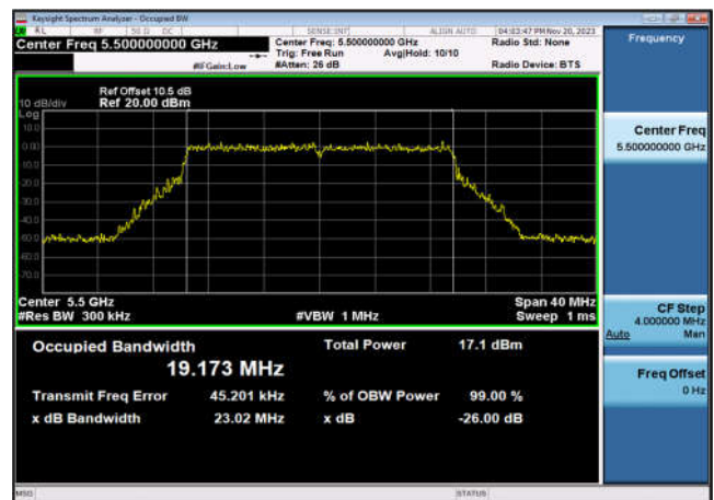
U-NII-2c 99% Bandwidth-802.11ax(20MHz ,5580MHz,Ant10
