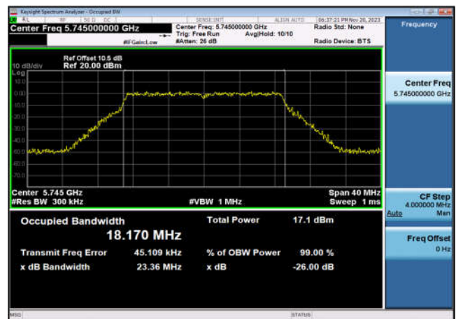
U-NII-3 99% Bandwidth-802.11ac(20MHz) ,5785MHz,Ant10
