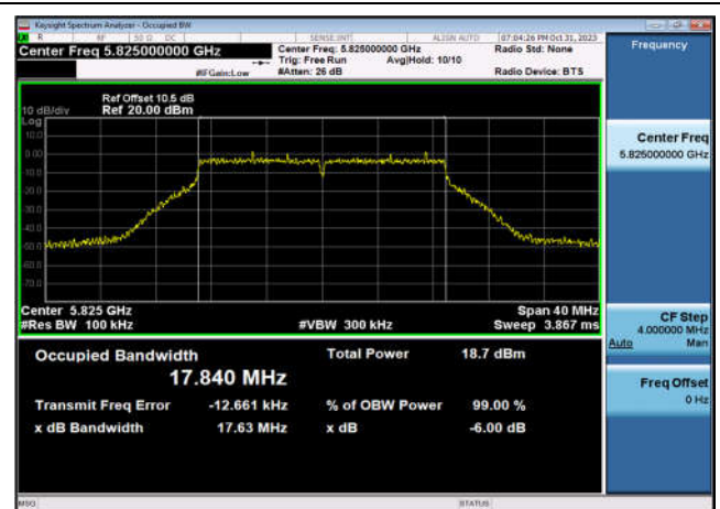
U-NII-3 6dB Bandwidth-802.11n(20MHz) ,5825MHz,Ant10
