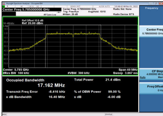
U-NII-3 6dB Bandwidth-802.11a(20MHz) ,5825MHz,Ant9
