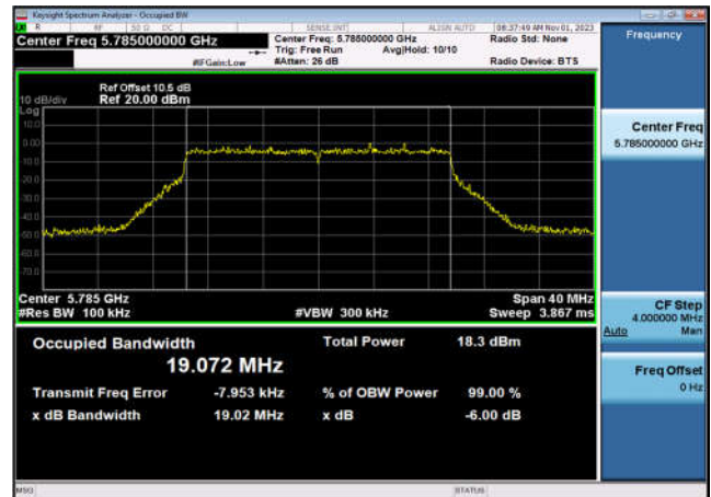
U-NII-3 6dB Bandwidth-802.11ax(20MHz) ,5825MHz,Ant10
