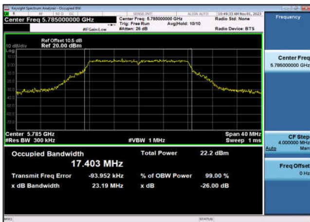
U-NII-3 99% Bandwidth-802.11a(20MHz) ,5825MHz,Ant9
