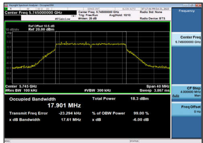
U-NII-3 6dB Bandwidth-802.11ac(20MHz) ,5745MHz,Ant10
