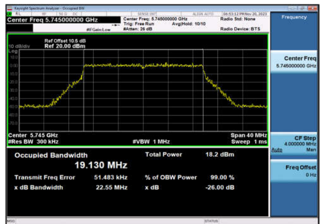
U-NII-3 99% Bandwidth-802.11ax(20MHz) ,5785MHz,Ant10
