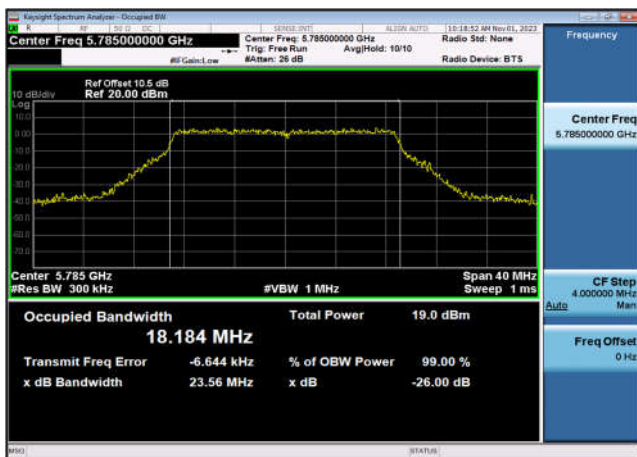
U-NII-3 99% Bandwidth-802.11ac(20MHz) ,5825MHz,Ant9
