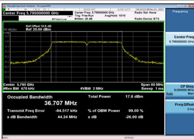
U-NII-3 99% Bandwidth-802.11n(40MHz) ,5795MHz,Ant9
