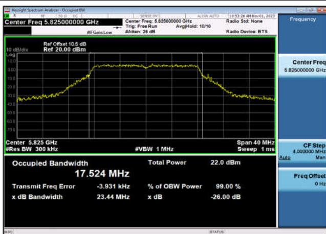
U-NII-3 99% Bandwidth-802.11a(20MHz) ,5825MHz,Ant9
