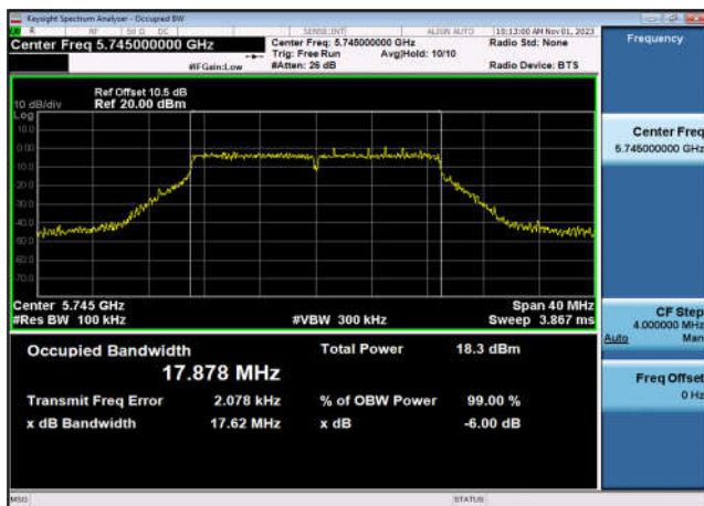
U-NII-3 6dB Bandwidth-802.11ac(20MHz) ,5745MHz,Ant9
