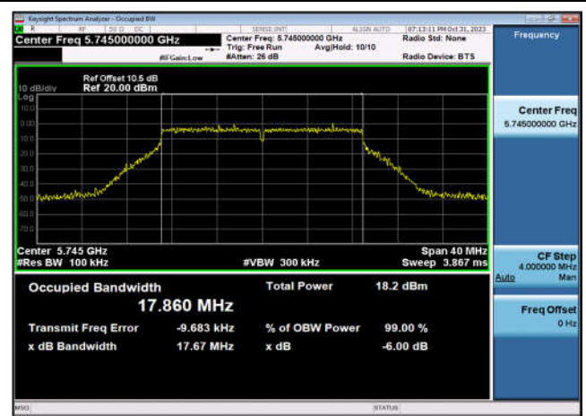
U-NII-3 6dB Bandwidth-802.11n(20MHz) ,5785MHz,Ant10
