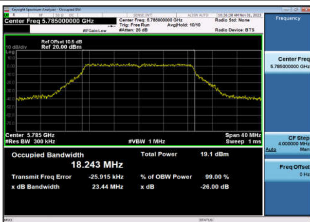
U-NII-3 99% Bandwidth-802.11n(20MHz) ,5785MHz,Ant9
