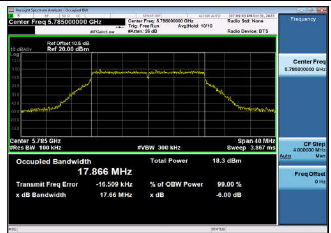
U-NII-3 6dB Bandwidth-802.11n(20MHz) ,5825MHz,Ant10
