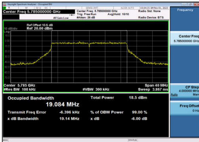
U-NII-3 6dB Bandwidth-802.11ax(20MHz) ,5825MHz,Ant9
