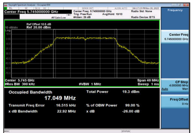
U-NII-3 99% Bandwidth-802.11a(20MHz) ,5785MHz,Ant10
