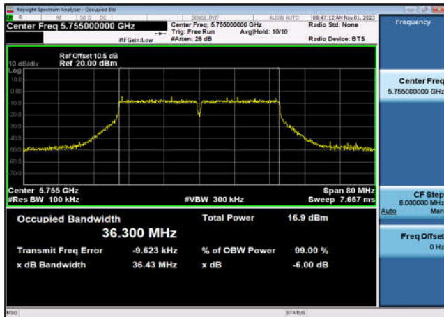
U-NII-3 6dB Bandwidth-802.11n(40MHz) ,5795MHz,Ant9
