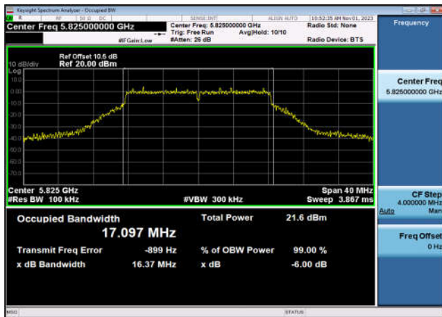
U-NII-3 6dB Bandwidth-802.11ac(20MHz) ,5745MHz,Ant9
