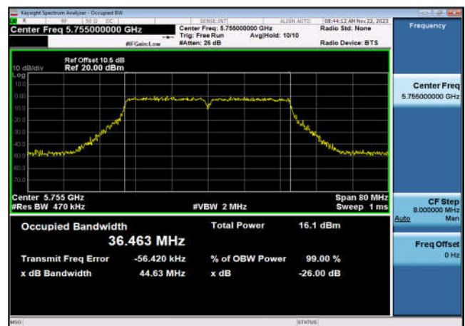
U-NII-3 99% Bandwidth-802.11n(40MHz) ,5795MHz,Ant10
