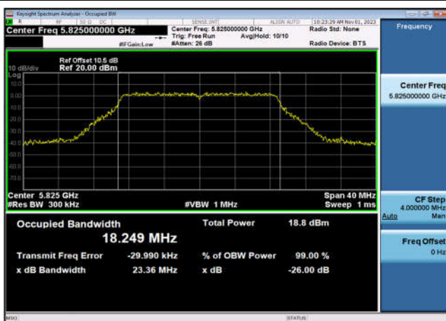
U-NII-3 99% Bandwidth-802.11ac(20MHz) ,5825MHz,Ant9
