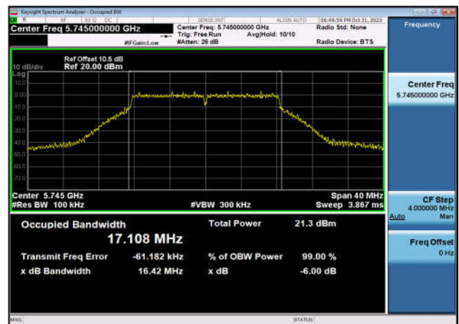
U-NII-3 6dB Bandwidth-802.11a(20MHz) ,5745MHz,Ant10
