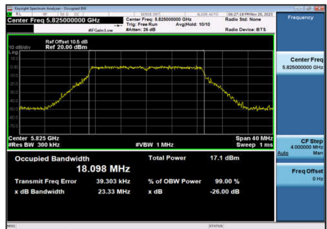
U-NII-3 99% Bandwidth-802.11n(40MHz) ,5755MHz,Ant10
