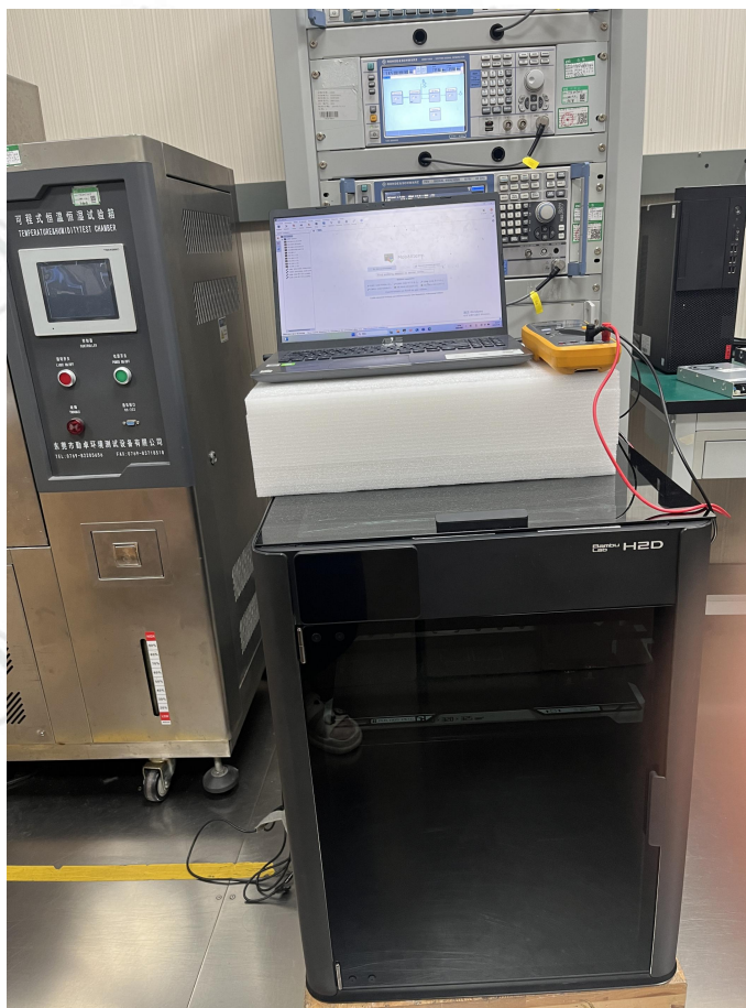
Radiated spurious emission Test Setup-1(Below 1GHz)
