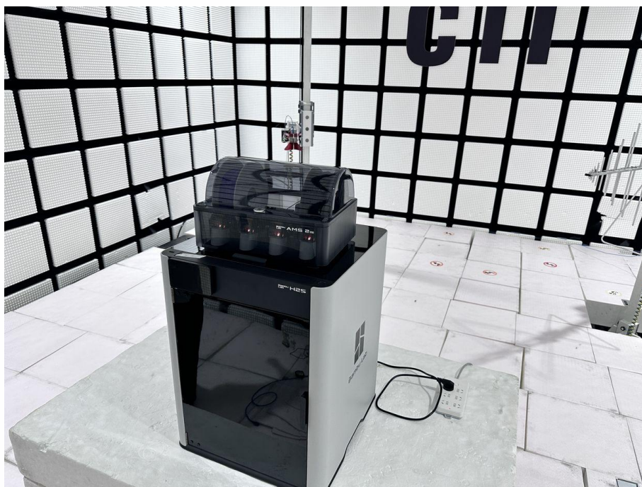
Radiated spurious emission Test Setup-2(Above 1GHz)
