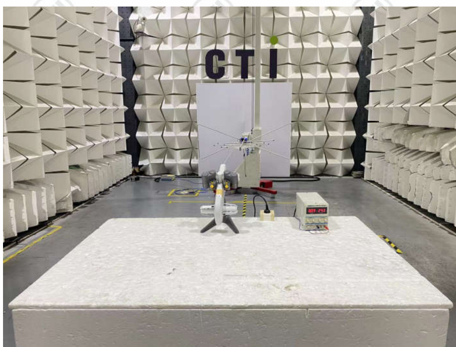
Radiated Spurious Emissions Test Setup (30MHz~1GHz)
