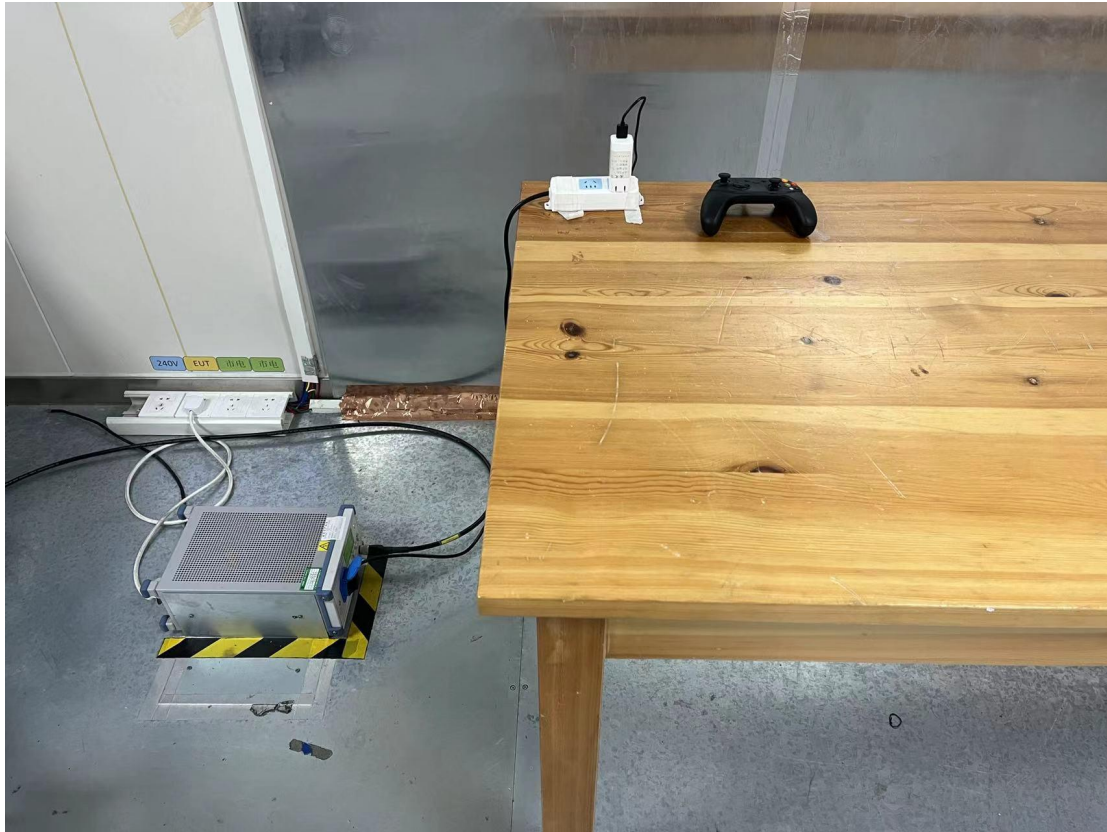
Conducted emission test setup
