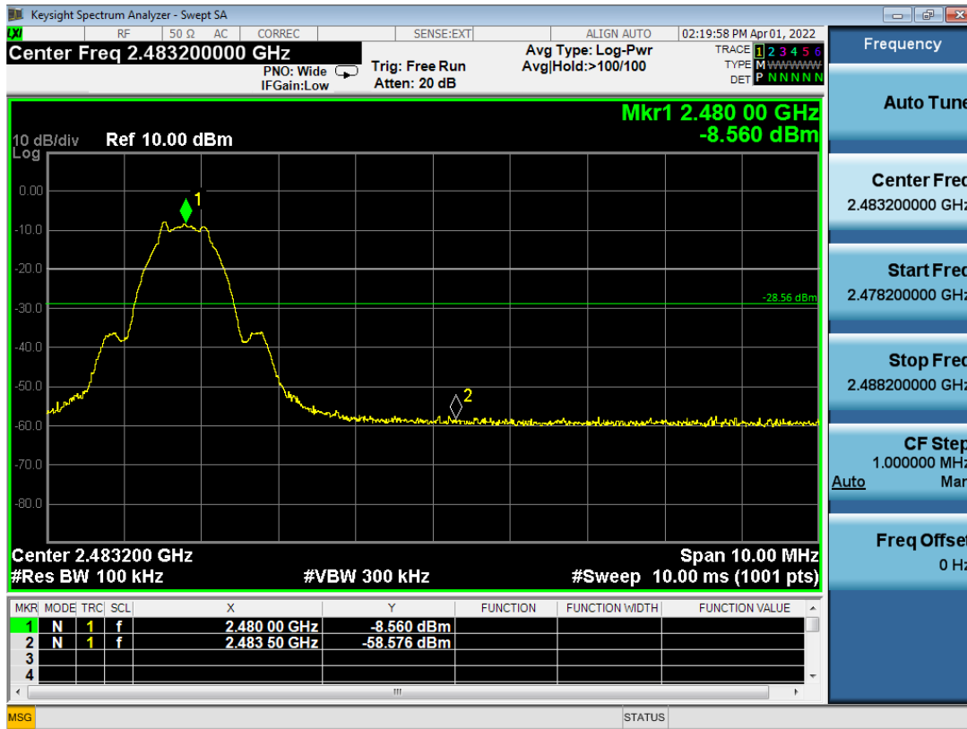
Figure 29: Emission on the Band Edge (High Channel)
