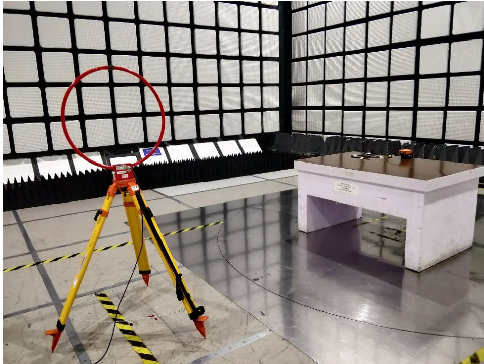
Figure 3: Photograph of RE test setup from 9 kHz to 30 MHz _ Perpendicular to EUT
