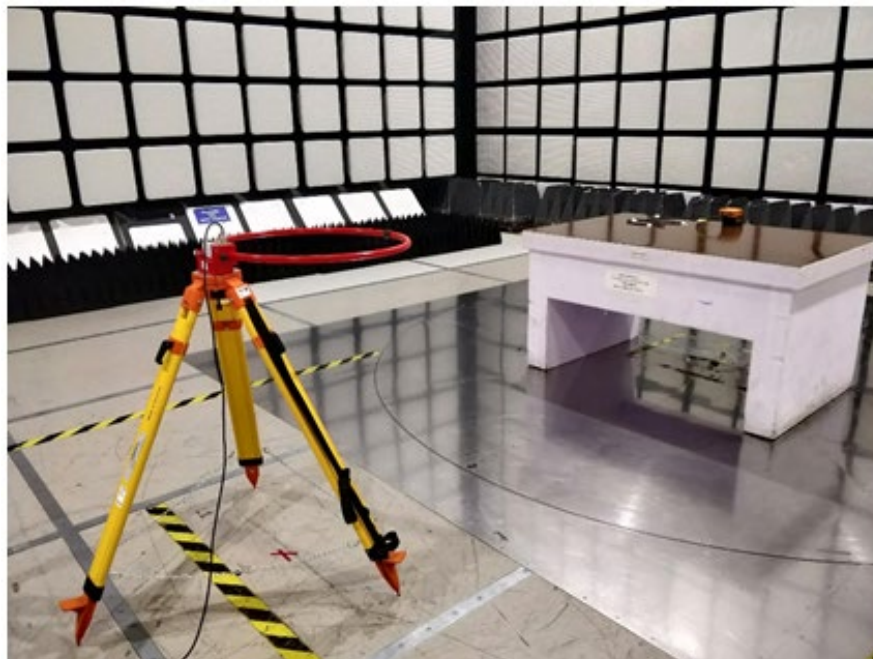
Figure 2: Photograph of RE test setup from 9 kHz to 30 MHz _ Parallel to Ground
