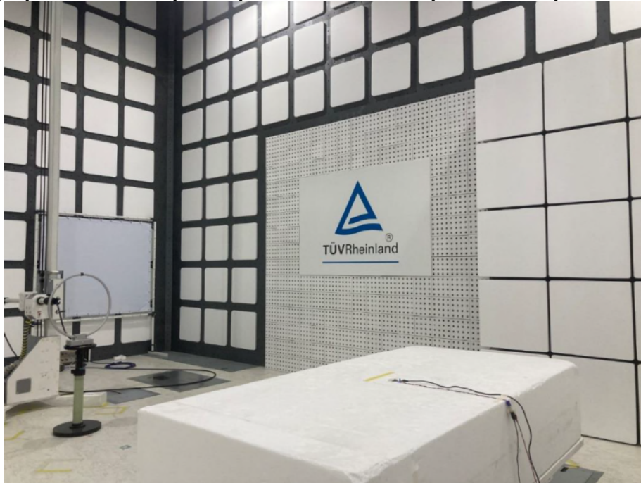
Photograph 3: Test Setup for Spurious Emissions (Back View 1)
