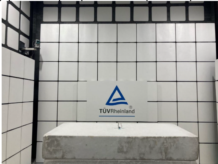
Photograph 2: Test Setup for Spurious Emissions (Front View 2)
