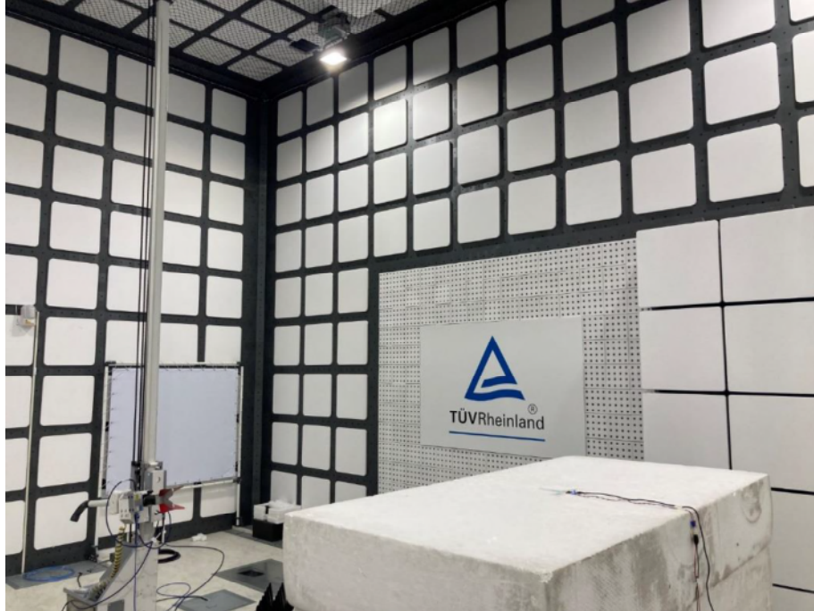
Photograph 5: Test Setup for Spurious Emissions (Back View 3)
