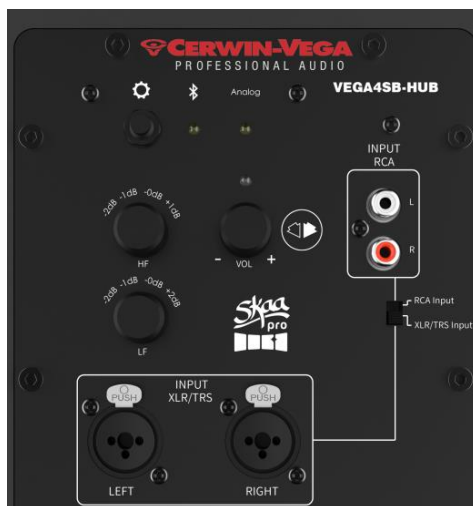
Figure 6: Direct Wired Input Connections
