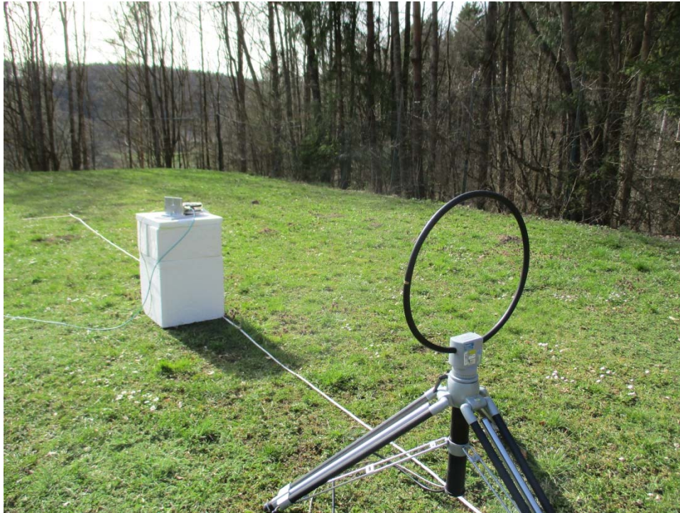
Photograph A1-5: Test site correlation for H Field Measurement in open field site at 3 m distance
