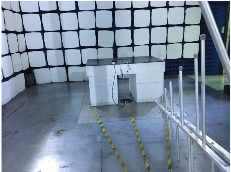
Radiation Emission Test Setup (30MHz to 1GHz)
