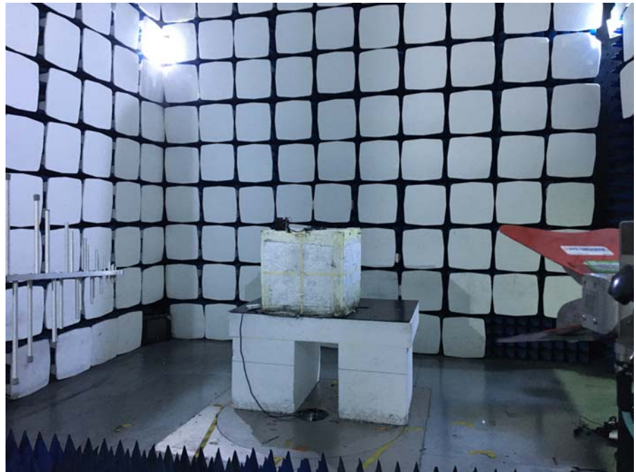
Radiation Emission Test Setup (1GHz to 18GHz)
