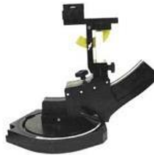
Figure 2 Device holder supplied by SPEAG
