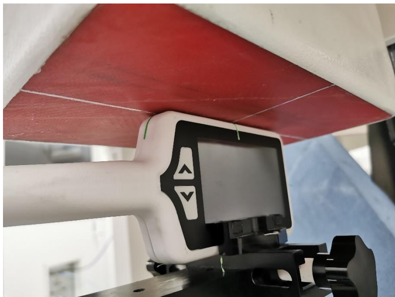
Figure 5. Left side of the DUT, 0mm separation distance
