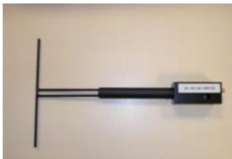
Figure 1 – Satimo COMOSAR Validation Dipole
