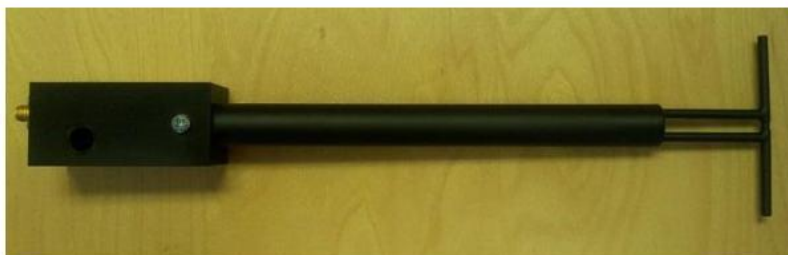
Figure 1 – MVG COMOSAR Validation Dipole
