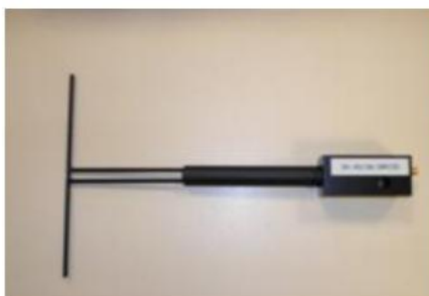
Figure 1 – Satimo COMOSAR Validation Dipole
