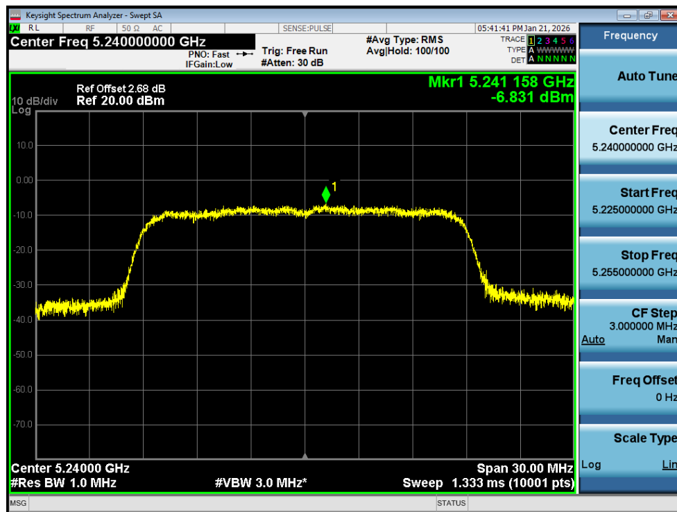
PSD NVNT n20 5240MHz Ant1
