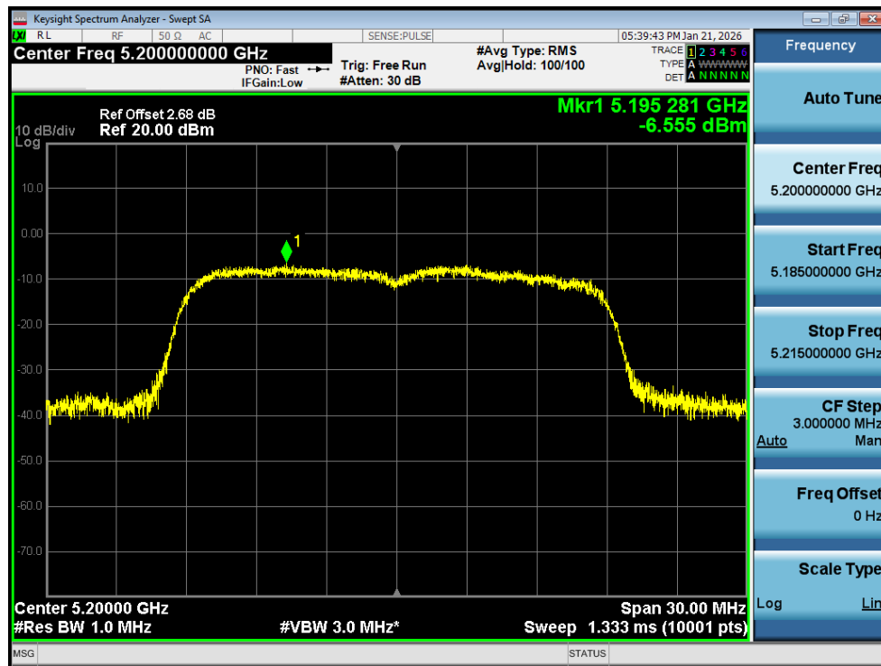
PSD NVNT n20 5200MHz Ant1
