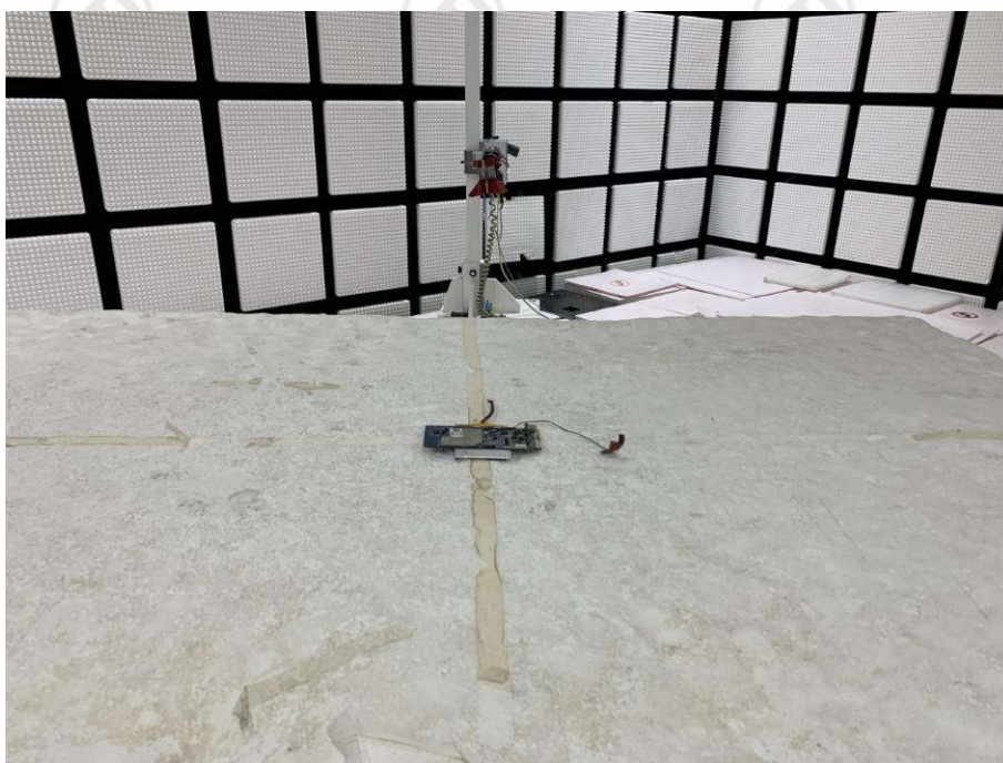
Radiated spurious emission Test Setup-2(Above 1GHz)
