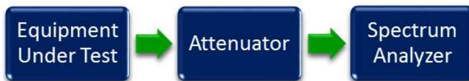
Figure 3. RF Power Test Setup
