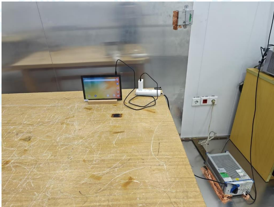
Photo of Setup for Conducted Emission
