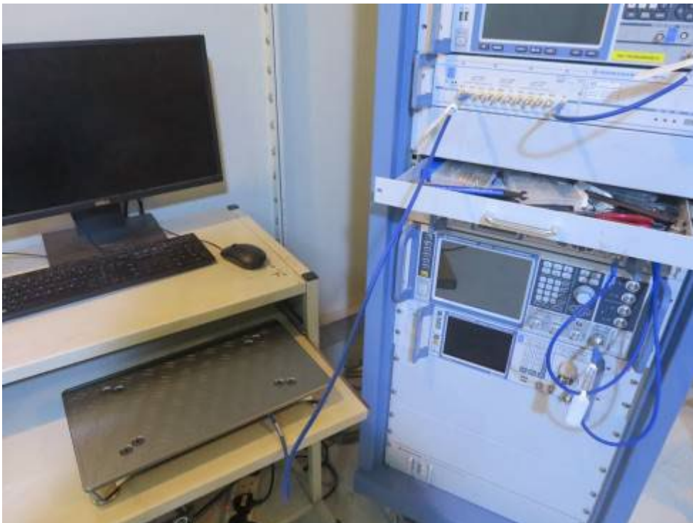
Conducted RF Output Power Test Setup
