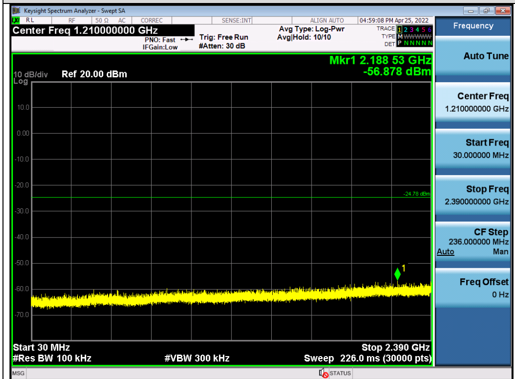
Test_Graph_BR_ANT1_2402_1Mbps_Lower Band Emissions
