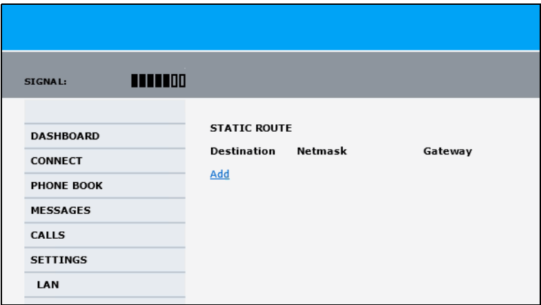
Figure 6-52: Web interface, Settings, LAN, Static route
