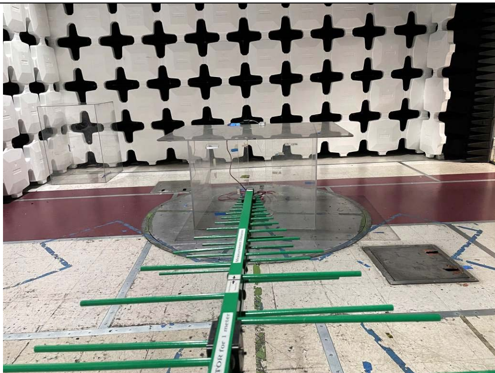
Radiated Emission Test below 30MHz Front View
