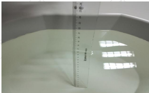
The Body Liquid of 750MHz (16.5cm)
