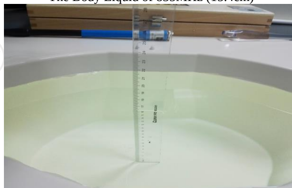
The Body Liquid of 1900MHz (16.4 cm)
