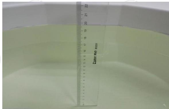
The Body Liquid of 835MHz (15.4cm)
