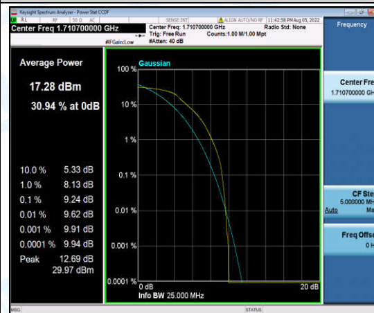
Band4-1.4MHz-16QAM-19957-6-0-Low-9.24-<=13-PASS
