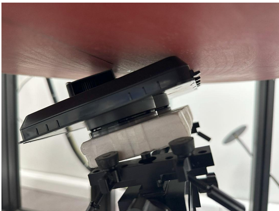
SAR Test Setup Photo 2 – NFC Body, Back Side at 0mm
