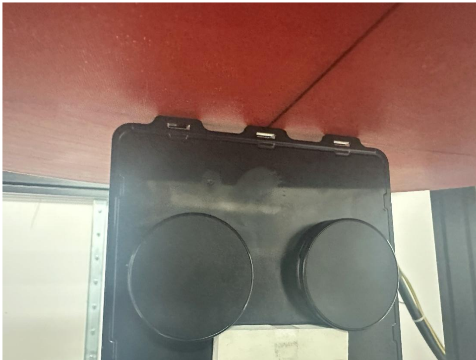
SAR Test Setup Photo 3 – NFC Body, Top Side at 0mm
