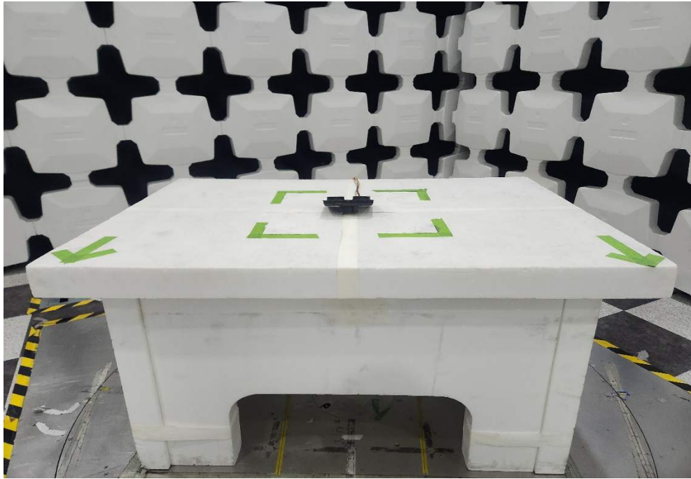
Figure 1. Test Setup – 9kHz-1GHz
