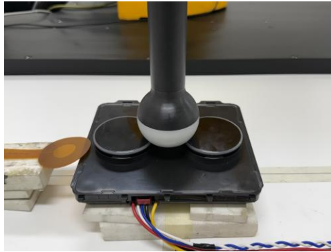
Test Setup Photo 1 Standby (Ping) Signal, Front side, 0mm
