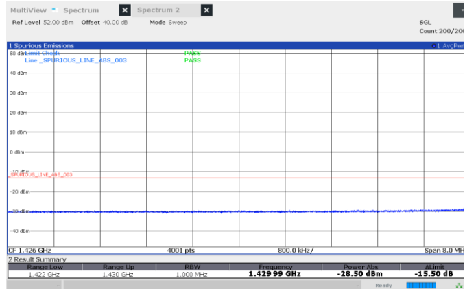
Figure 8.5-12: Spurious emissions at antenna terminals, Band Edge-2, Low CH 1433 MHz, 0.05 MHz, CPM
