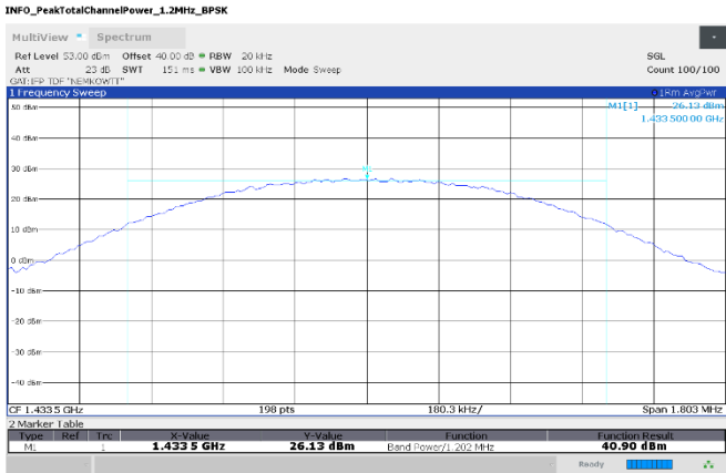
Figure 8.4-9: Output power, Mid CH 1433.5 MHz, 1.2 MHz, CPM
