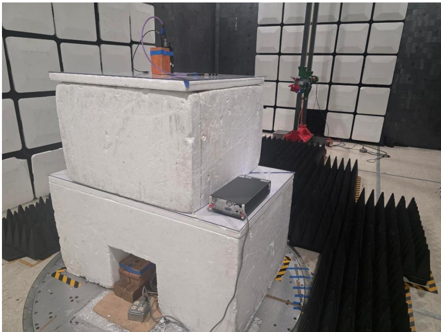
Figure 8 - Radiated emissions above 1 GHz (1 – 18 GHz), rear view (50kHz BW with GNSS Simulator)
