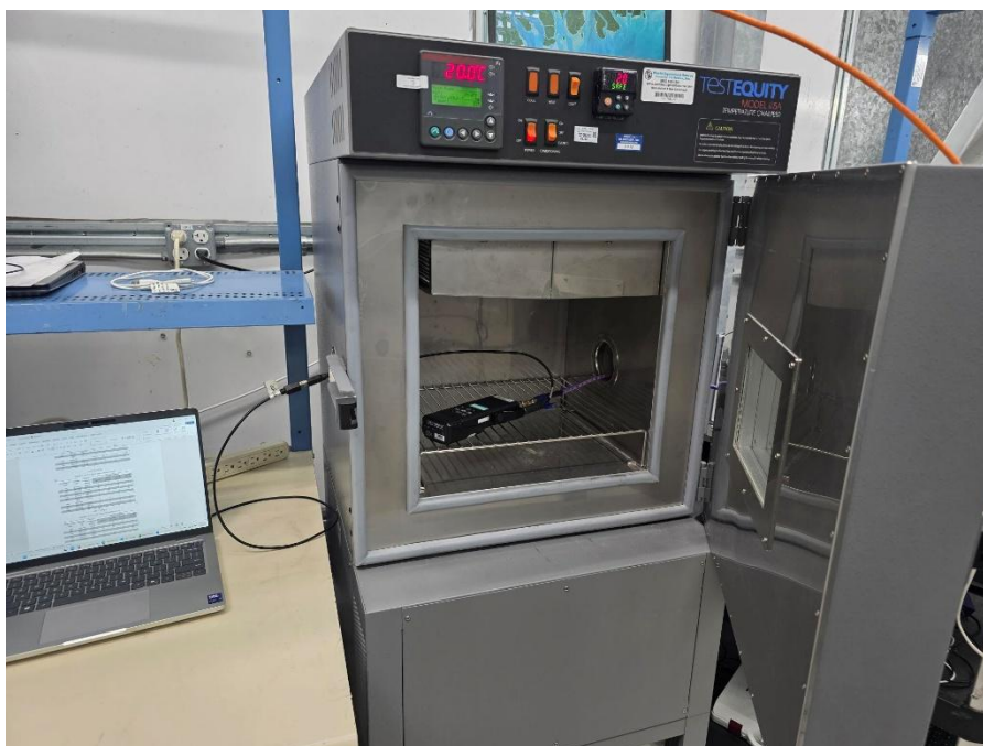
Figure 12 – Test setup (Frequency stability)
