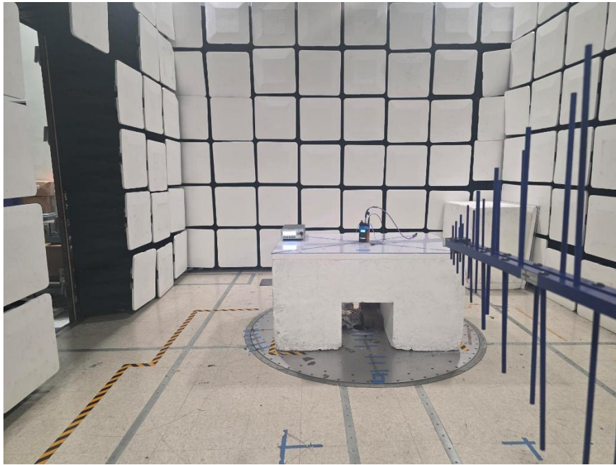
Figure 3 - Radiated emissions below 1 GHz (0.03 – 1 GHz), front view (50kHz BW with GSNN Simulator)
