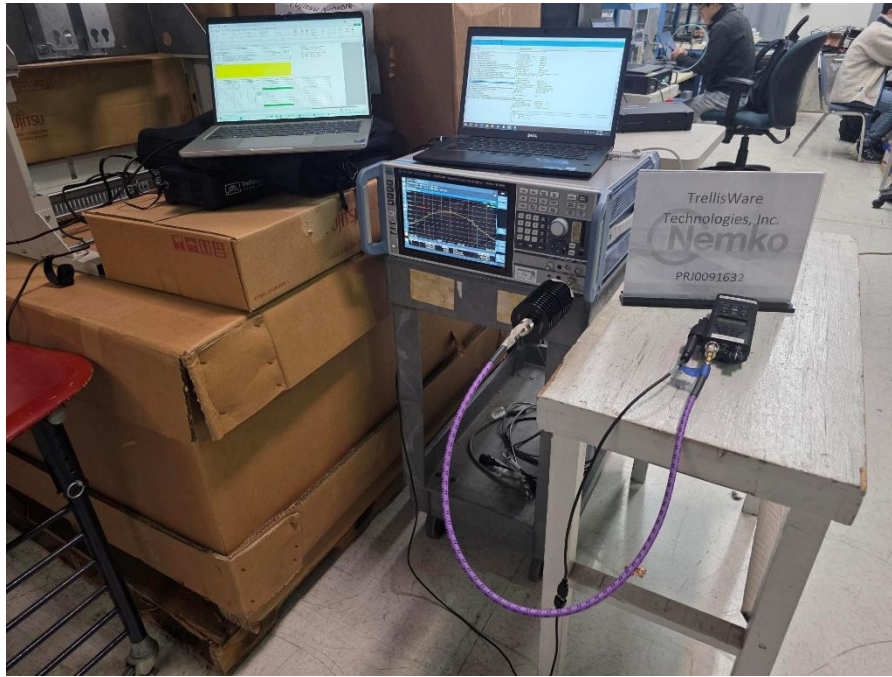
Figure 9 – Test setup (spectrum analyzer measurements)
