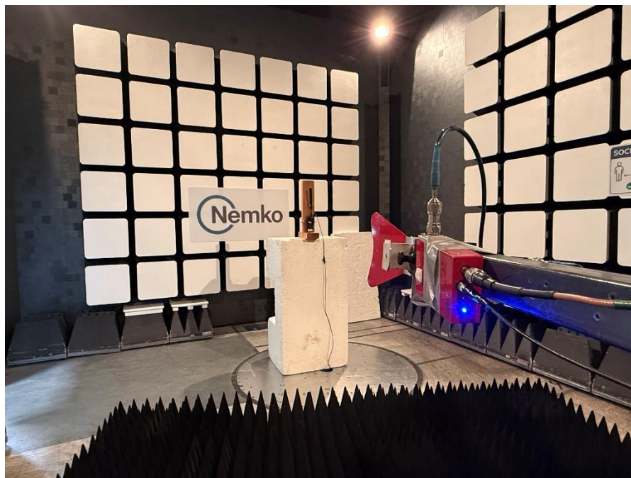
Figure 7.3-15: Radiated spurious emissions – above 1 GHz
