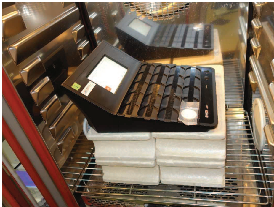
Photograph 5: Set-up for Frequency Stability, inside Temperature Chamber
