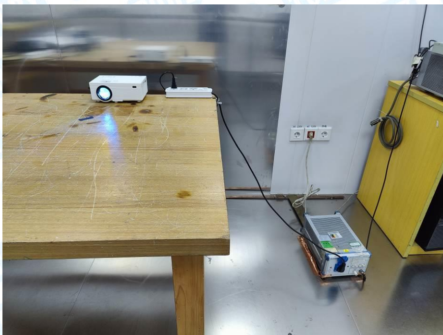
Photo of Setup for Conducted Emission
