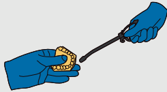
⑤ Dry parts with compressed air
