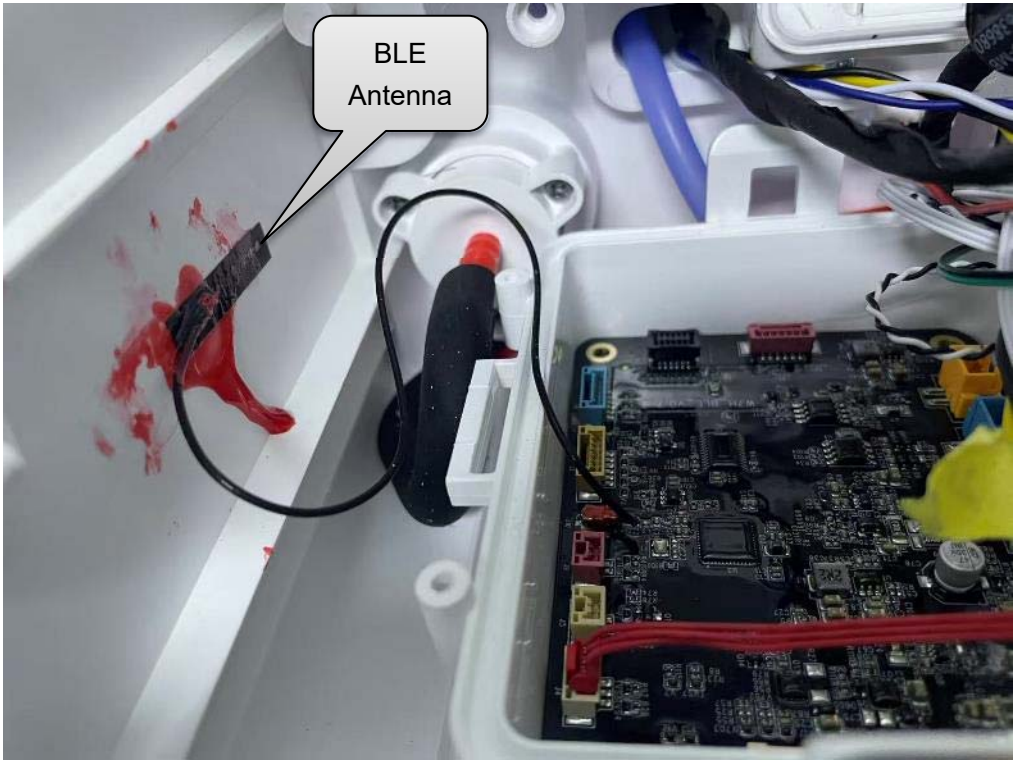
Bluetooth Antenna position
