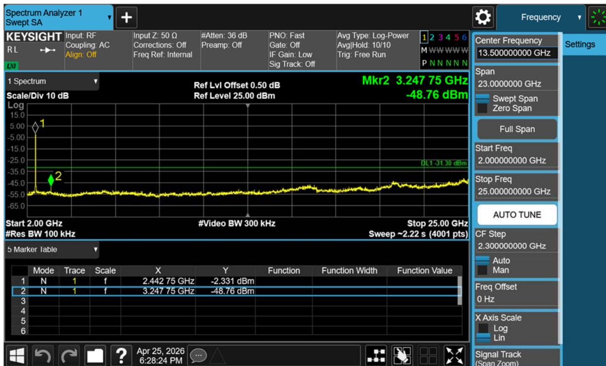
Figure 37: Conducted Spurious Emission & Authorized-band band-edge, 802.11n(HT20), 2462MHz Carrier Level
