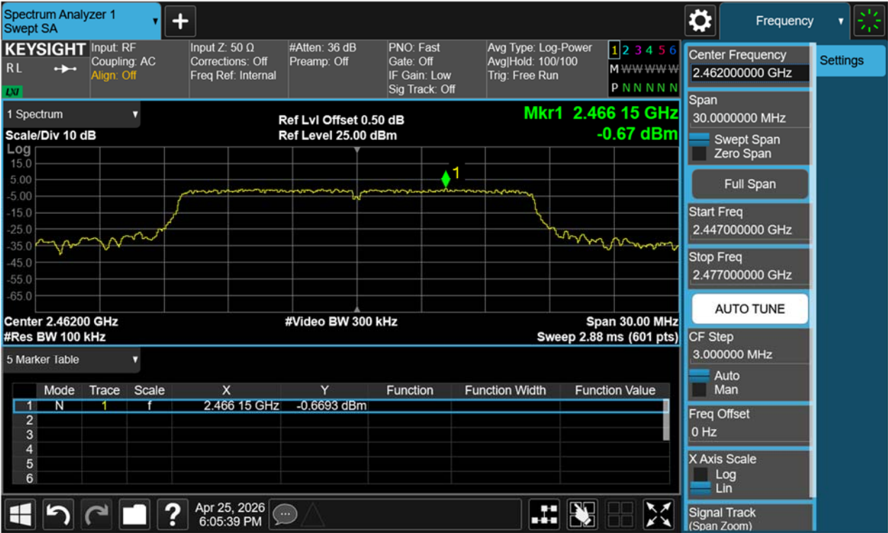
Figure 34: Conducted Spurious Emission & Authorized-band band-edge, 802.11g, 2462MHz Carrier Level
