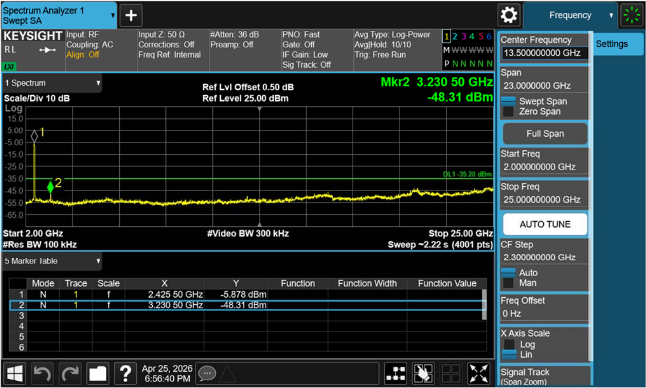
Figure 39: Conducted Spurious Emission & Authorized-band band-edge, 802.11n(HT40), 2437MHz Carrier Level
