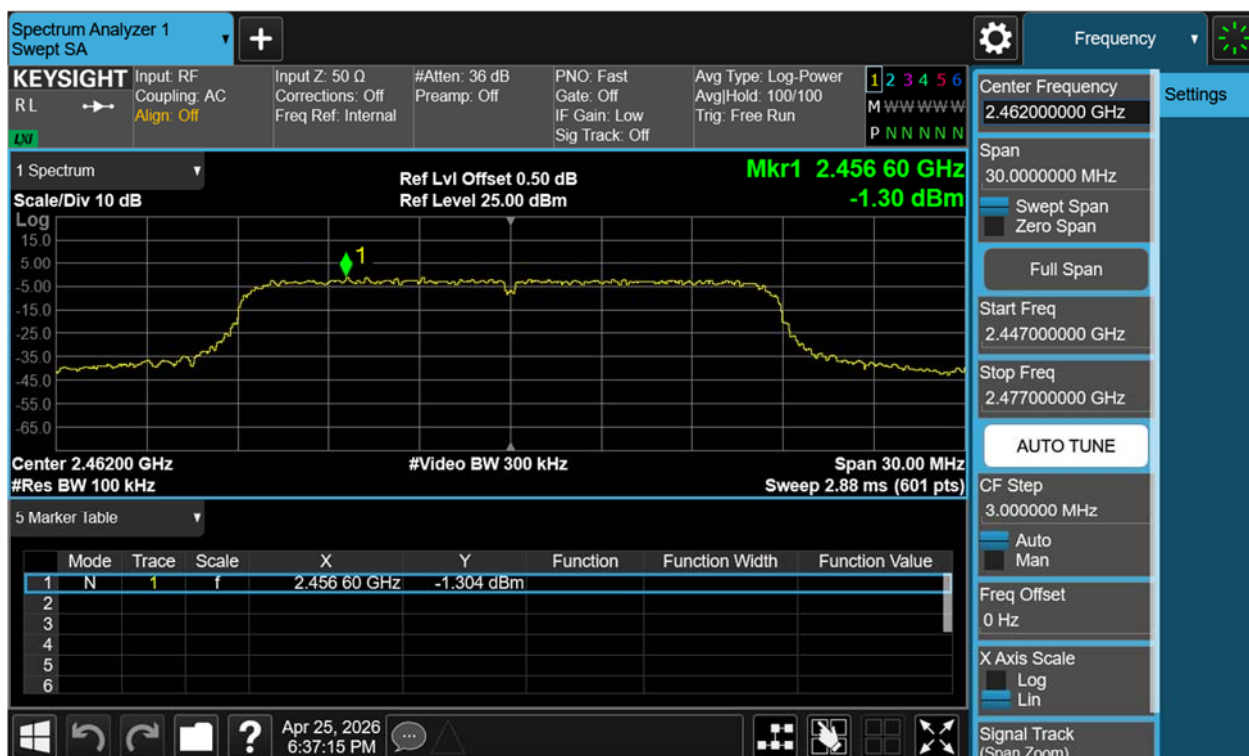
Figure 37: Conducted Spurious Emission & Authorized-band band-edge, 802.11n(HT20), 2462MHz Carrier Level
