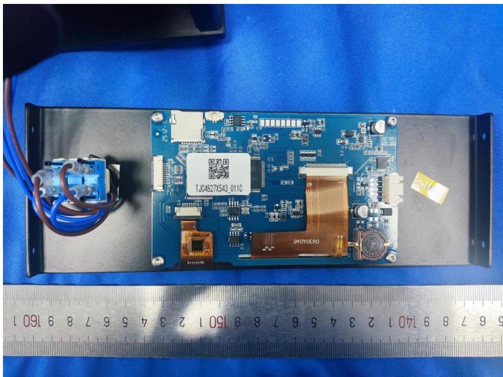
Photo 10: internal view for emergency switch and LCD module
