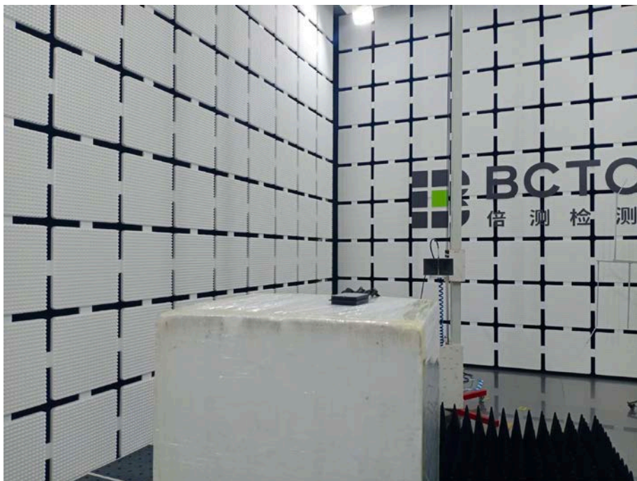
Spurious Emission Test Setup (Above 1GHz)
