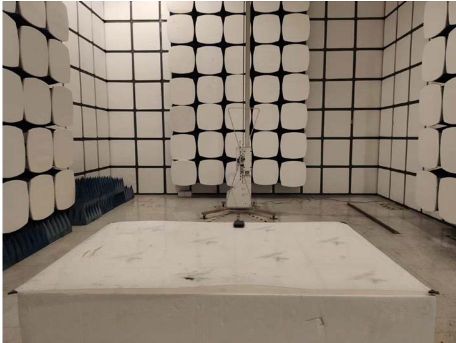
Spurious Emission Test Setup (Below 1GHz)
