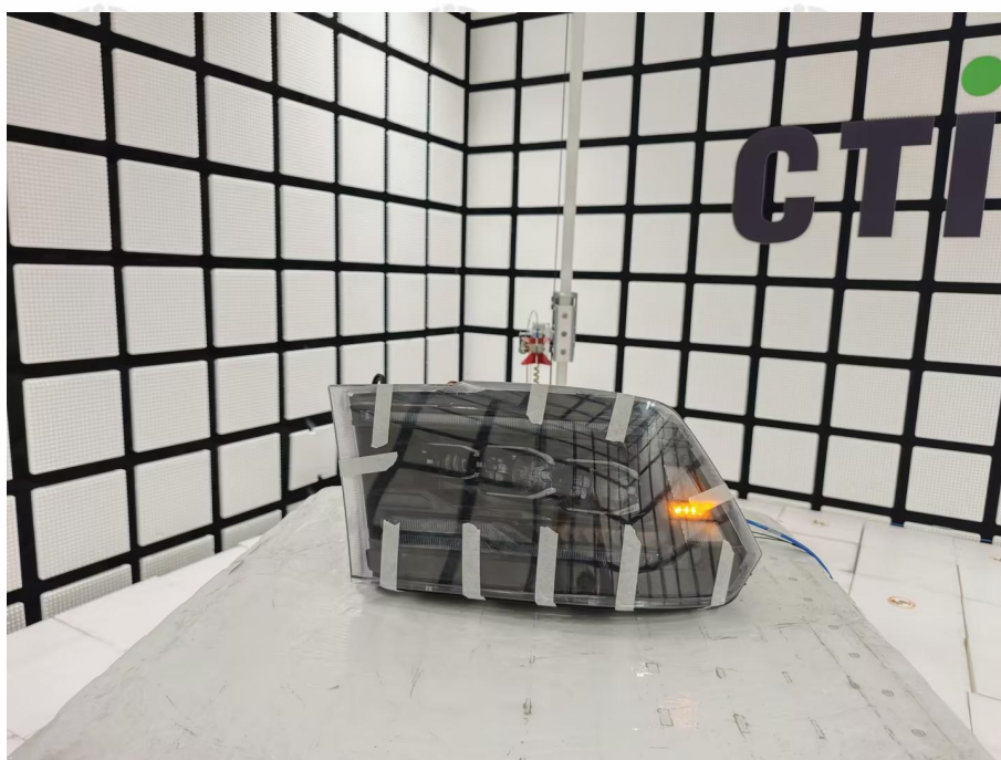
Radiated spurious emission Test Setup-2(Above 1GHz)
