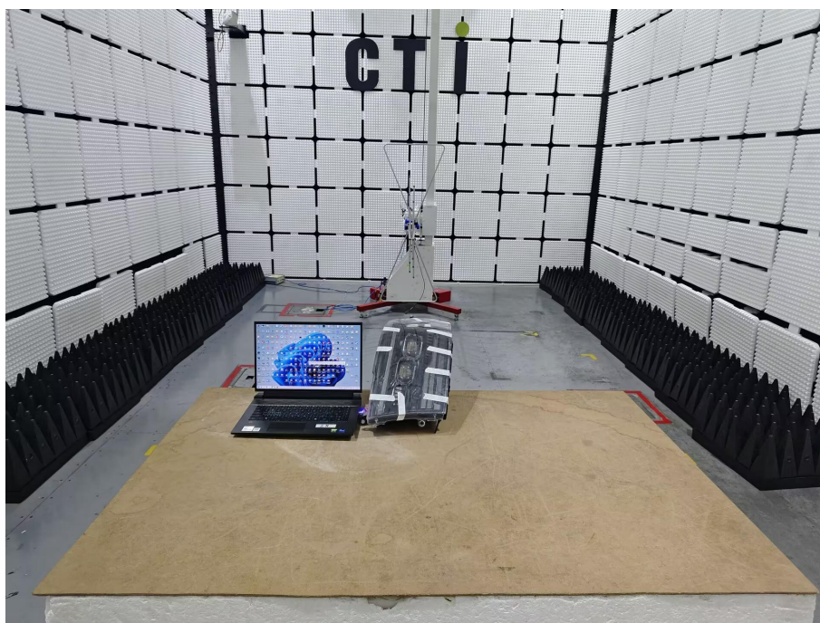
Radiated spurious emission Test Setup-1(Below 1GHz)
