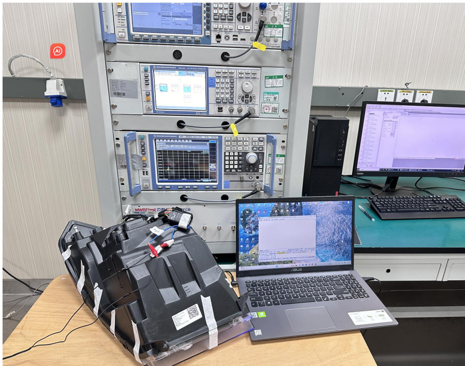
Conducted Emissions Test Setup-1
