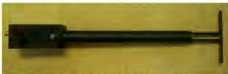
Figure 1 – MVG COMOSAR Validation Dipole
