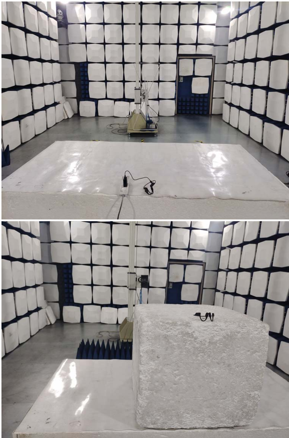
Radiated emission test view
