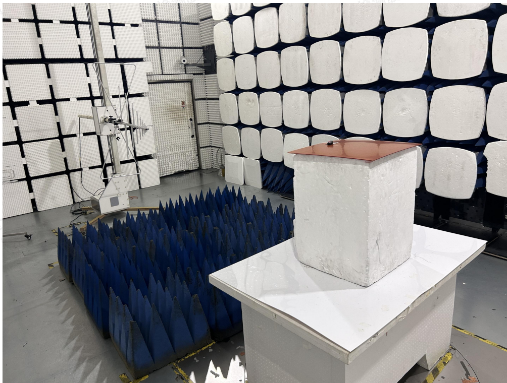
Radiated Emissions Measurement (Below 1GHz)
