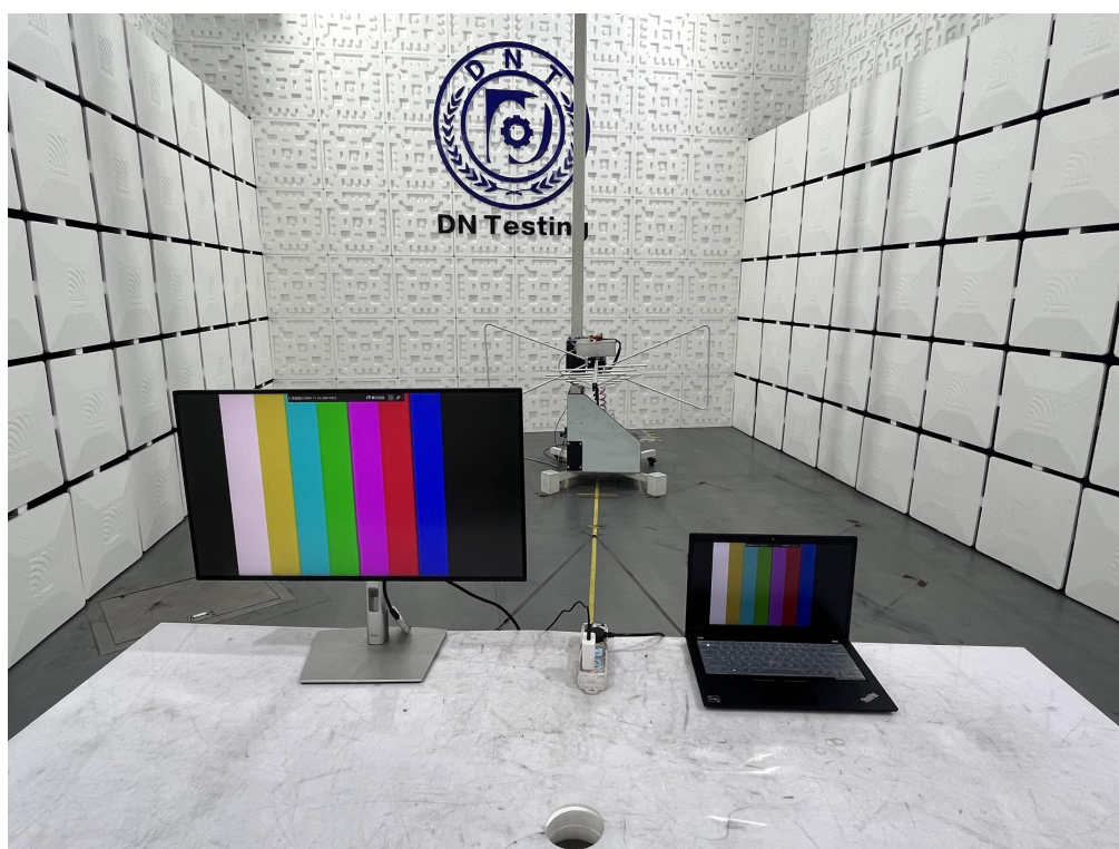
Radiated Emission Test View|(Below 1G)
